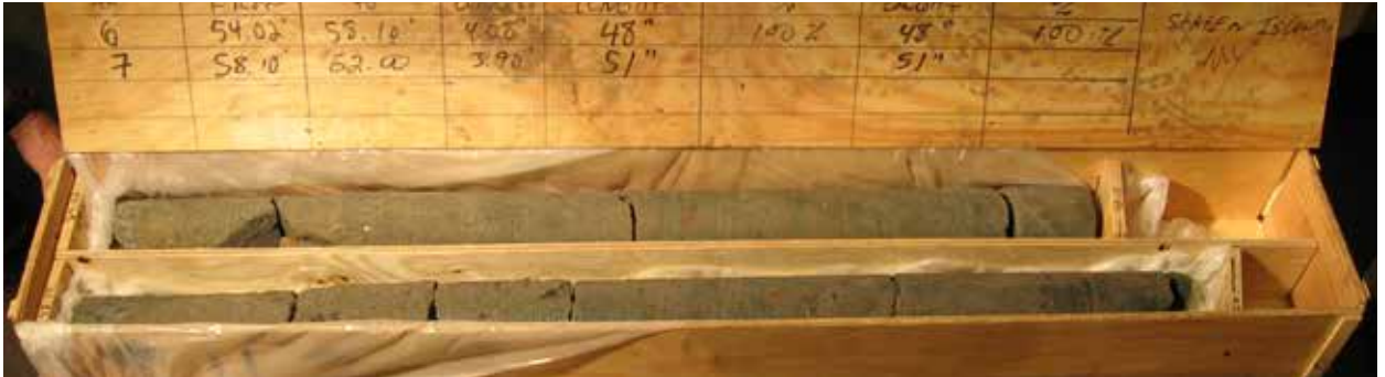
Fig. 11. Coring of fine alluvial deposit.
