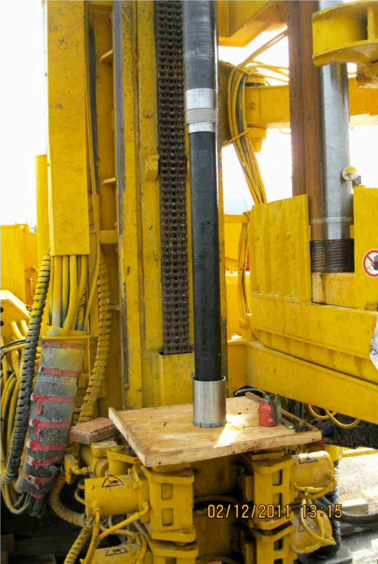
Fig. 10. Extraction of a perfect cored sample
