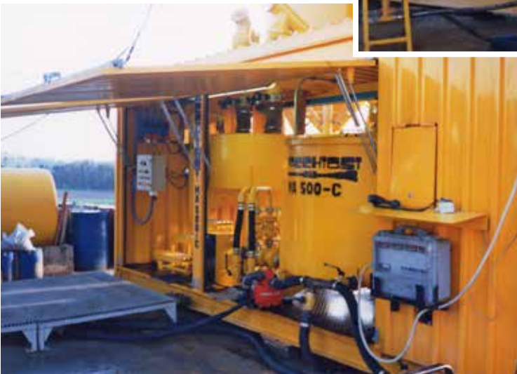
Fig. 10. MA 500 C mixer and PRS3 data acquisition instrument.
