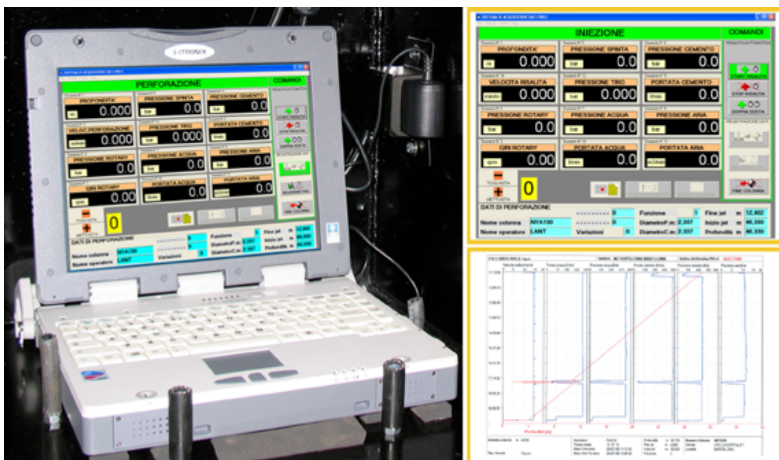
Fig. 10, - PRS3 data acquisition and recording system.
