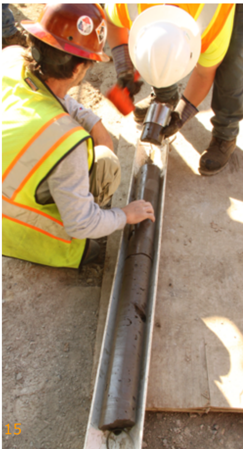
Fig. 15 | 16 | 17 - Checks carried out on the columns by means of core drilling.
