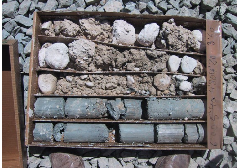
Fig. 2. Core samples from the area of interest, showing the two lithology types involved in the consolidation works.
