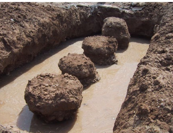
Fig. 3. Pictures of the test field columns. The significant amounts of water at the site are clearly visible.
