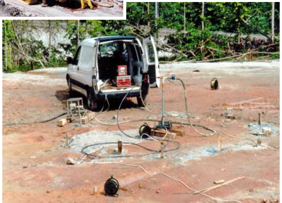
Fig. 6. Pumping test with measurement of the water table level.
