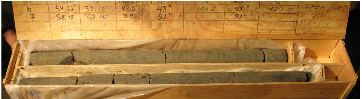
Fig. 11. Coring of fine alluvial deposit.
