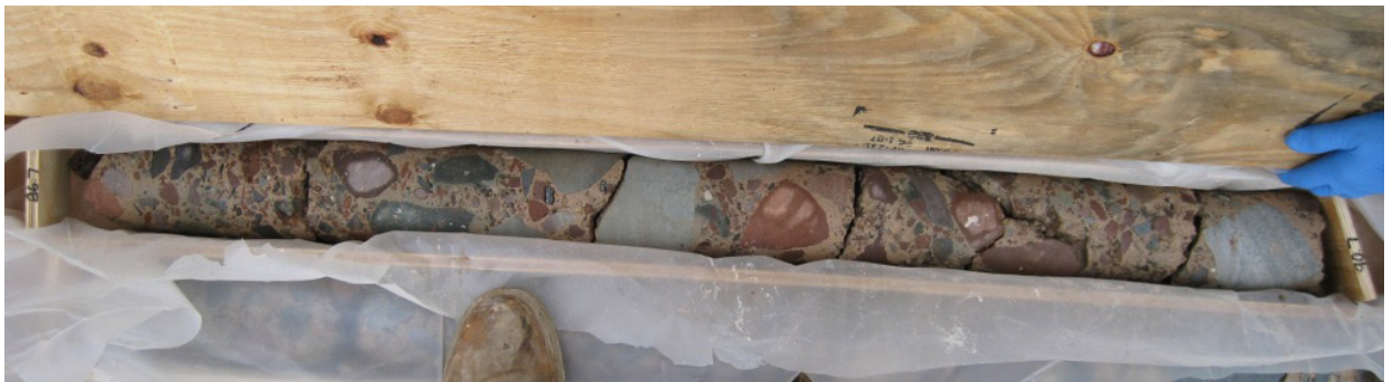
Fig. 12. Coring of grouted glacial deposit, with boulders and cobbles.
