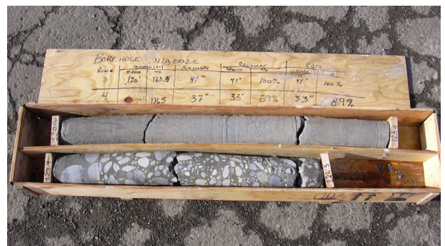
Fig. 3. View of the contact between the clay and gravel from core samples
